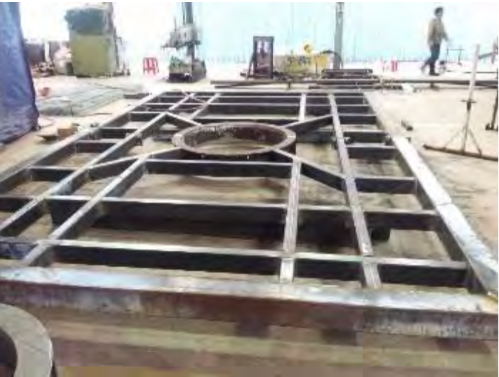
BOP WORKING PLATFORM – DESIGNED & BUILT FOR SEADRILL JACK-UP RIG WEST CRESSIDA & ROWAN DRILL JACK-UP RIG EXL 4
