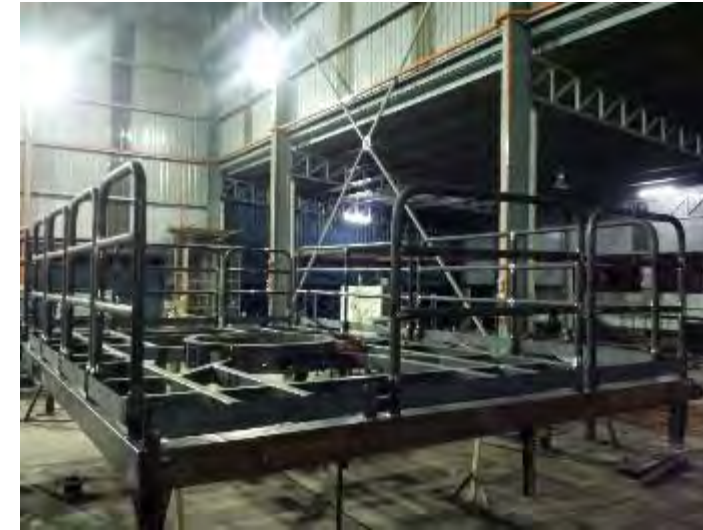
BOP WORKING PLATFORM – DESIGNED & BUILT FOR SEADRILL JACK-UP RIG WEST CRESSIDA & ROWAN DRILL JACK-UP RIG EXL 4
